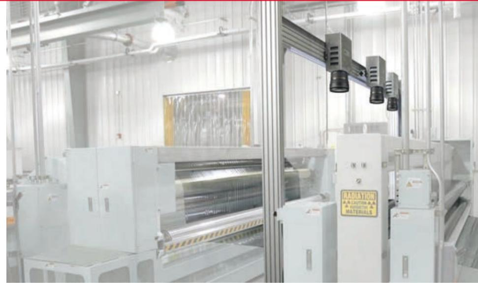
PET film extrusion with optical quality control system (source: OCS GmbH)
