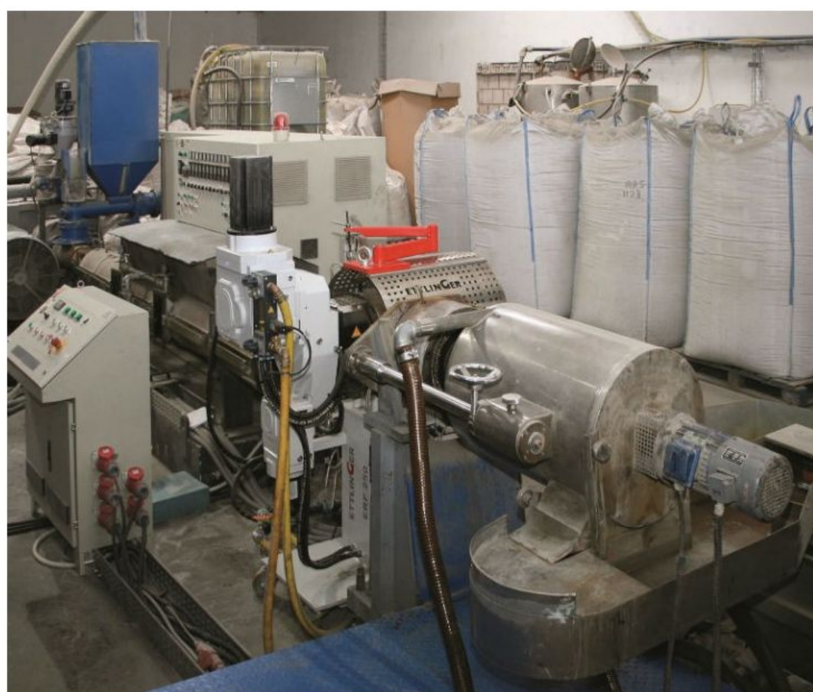
CPE Entsorgung GmbH uses an ERF melt filter from Ettliger Kunststoffmaschinen to recycle PS waste from end-of-life refrigerators into high-quality recycled material used to make foils for thermoformed products.
